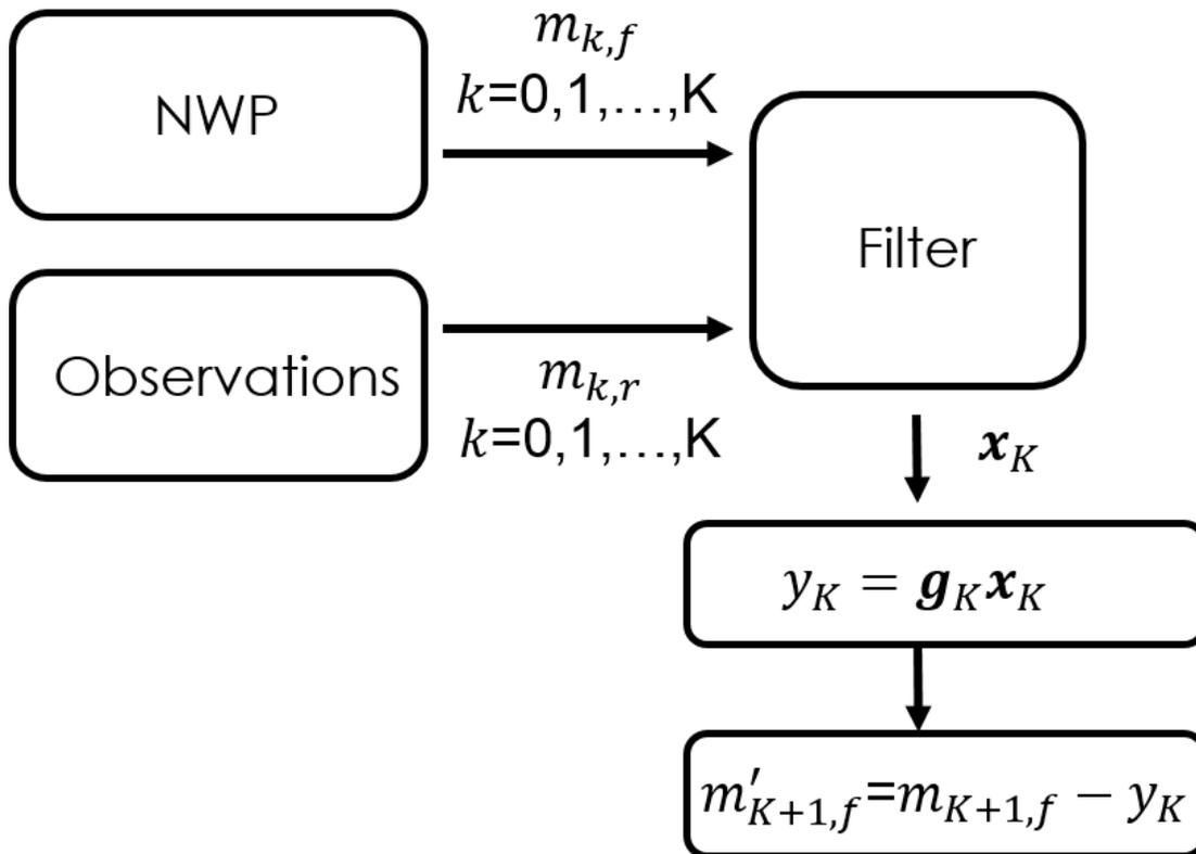
Fig. 1. Block diagram of post-processing by a filter such as the KF or  $H_\infty$  filter. An NWP output of  $m_{K+1,f}$  is corrected by  $y_K$ , and updated as  $m'_{K+1,f}$ .
